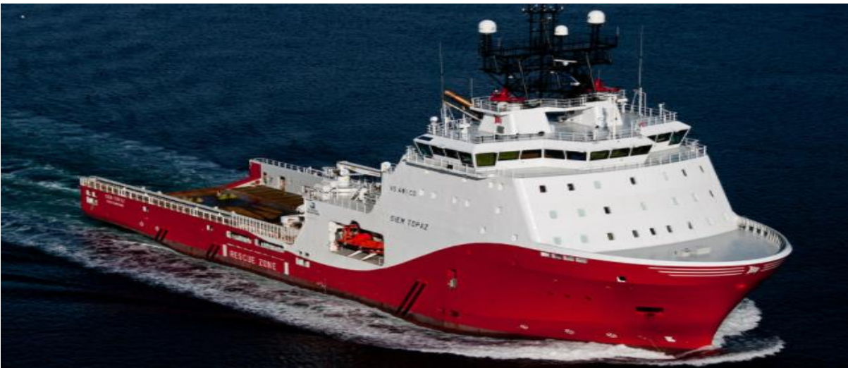
Figure 9: Example of an Anchor Handling Tug
