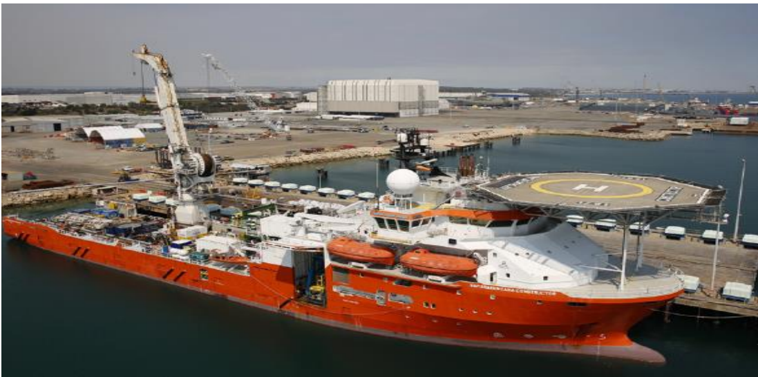
Figure 12: Example of an Installation Support Vessel/Dive Support Vessel
