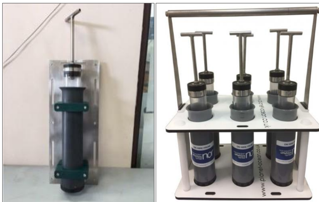
Figure 3-3 Raytech push corer and attachment plate (left) and milk crate style carrier (right)
