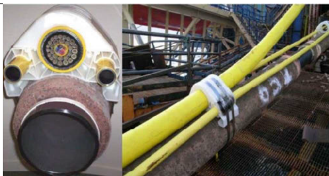
Figure 1: Minerva pipeline bundle and individual piggyback clamp components
