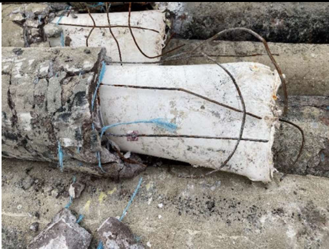
Figure 2: Recovered pipe section showing plastic inner lining, concrete coating and bailing twine
