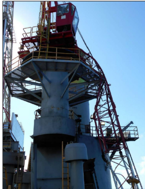
Crane boom collapse following failure of the luffing winch pawl - Nov 2017
