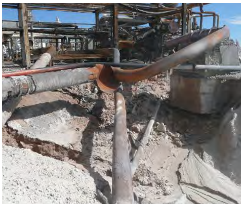
Ruptured 16 sales gas line: Photo from published NOPSA investigation report, October 2008
