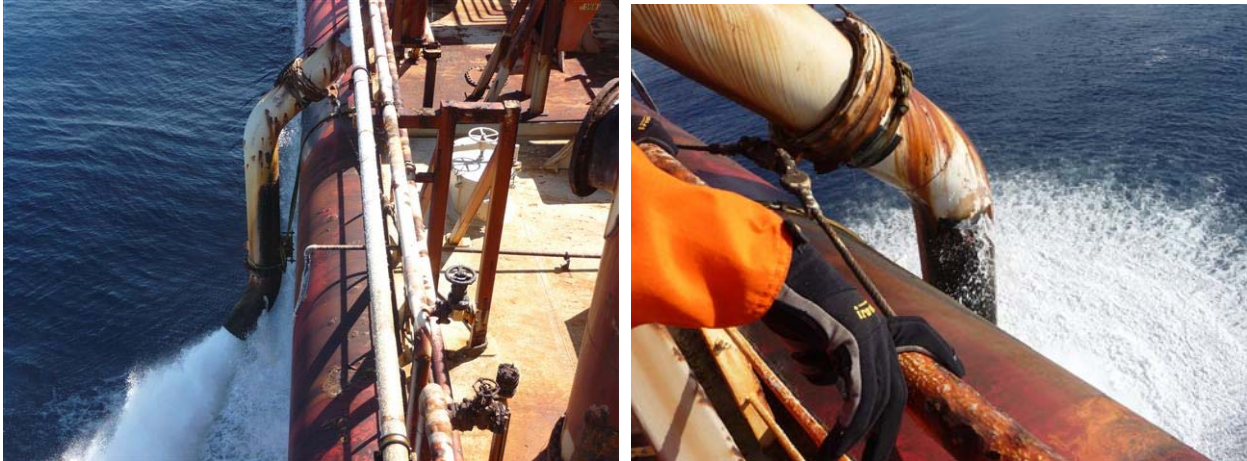
Figures 3 and 4 - Process Cooling SW Overboard Line
