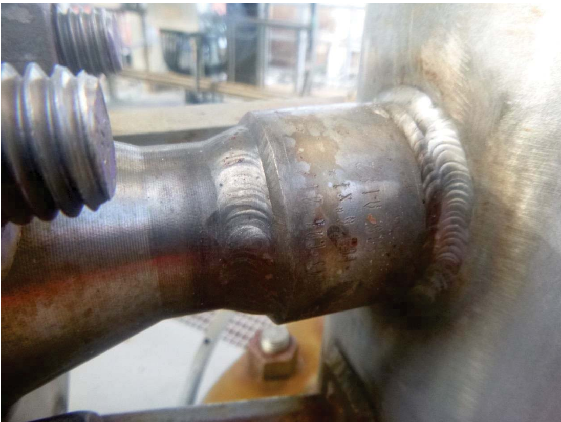
Figure 2 - 150-FG-4028-03D01-0 TP1 (B) condition of small bore fitting weld
