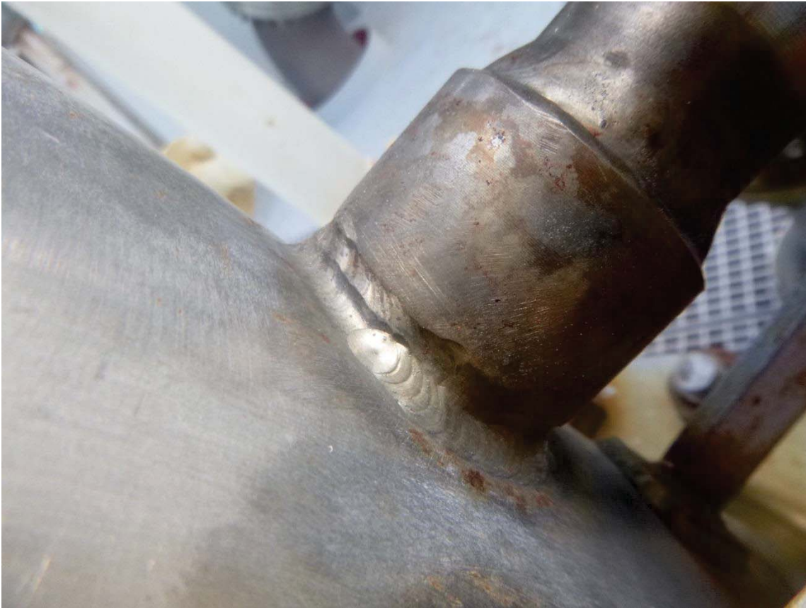
Figure 4 - 150-FG-4028-03D01-0 TP1 (B) condition of small bore fitting weld
