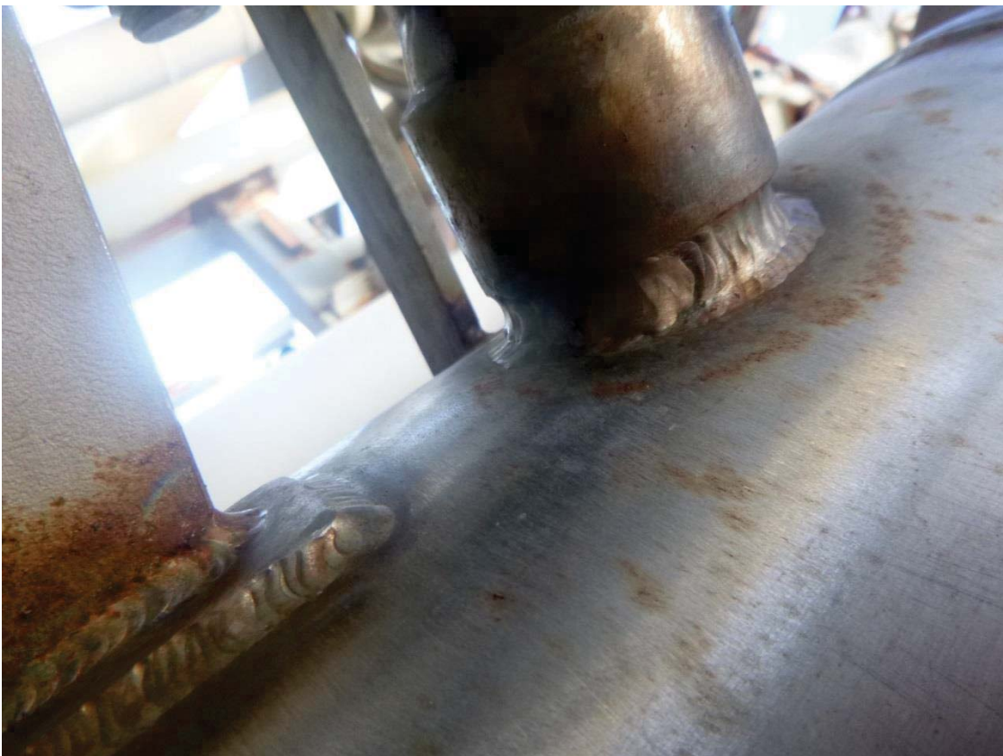
Figure 6 - 150-FG-4028-03D01-0 TP2 (A) condition of small bore fitting weld
