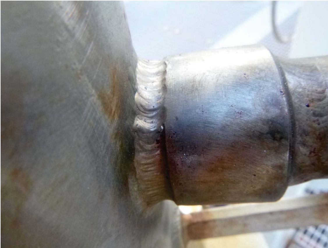
Figure 6 - 150-FG-4028-03D01-0 TP2 (A) condition of small bore fitting weld
