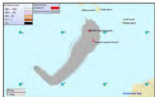
Figure 5: Predicted oil thickness on the sea surface at 10 and 19 hours and at 2, 4, and 5 days after the initial release (3:00 am, 7 th June 2010) for the worst case spill trajectory identified from the diesel scenario. Results are based on a 300 m 3 release of diesel over 6 hours, following a vessel spill incident during January to June wind and current conditions.
