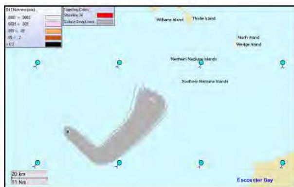
Figure 5: Predicted oil thickness on the sea surface at 10 and 19 hours and at 2, 4, and 5 days after the initial release (3:00 am, 7 th June 2010) for the worst case spill trajectory identified from the diesel scenario. Results are based on a 300 m 3 release of diesel over 6 hours, following a vessel spill incident during January to June wind and current conditions.
