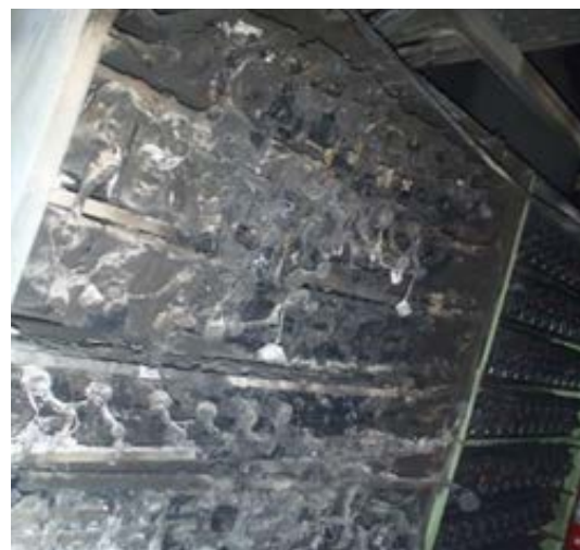
Figure 2 – Battery cabinet with doors removed. Damage within left cabinet.
