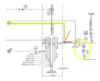
Figure 2 – Example P&ID drawing showing the instrument take-off point (arrow) incorrectly located downstream of the UV shutdown valve (circled).
