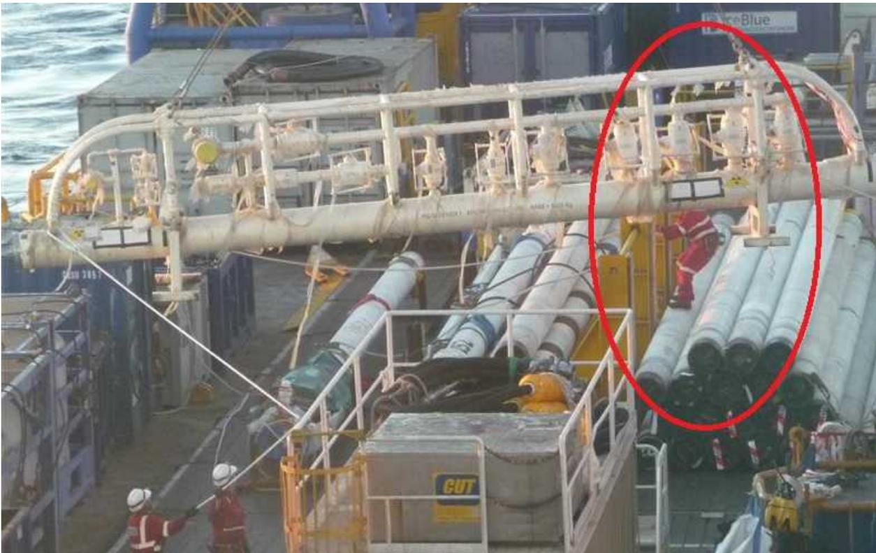
Accessibility refers to the ease with which an item can be accessed for manual operation, replacement, or maintenance. Items known to require manual operation or maintenance should be designed and located in such a way as to be accessible without the need to first remove items or equipment belonging to other
