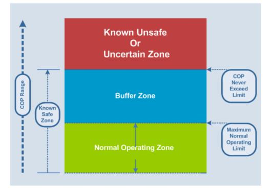
Figure 9 – Critical Operating Parameter zones
