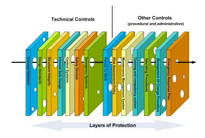
Figure 8 – Layers of Protection
