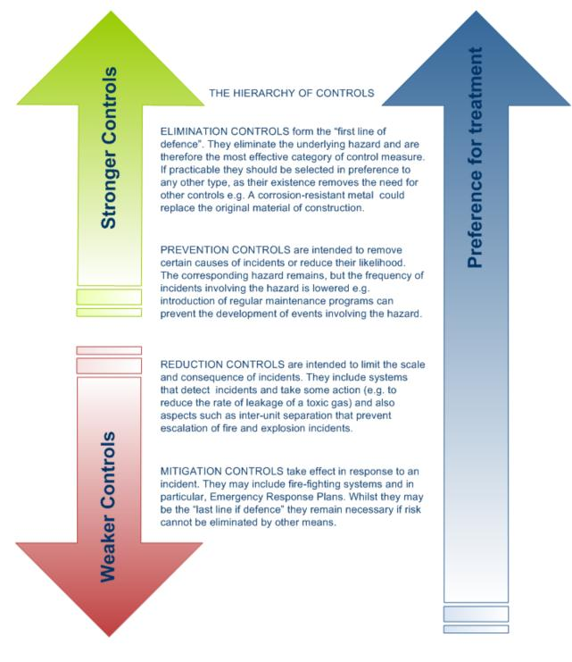
Figure 7 – Example of a Control Measure Hierarchy
