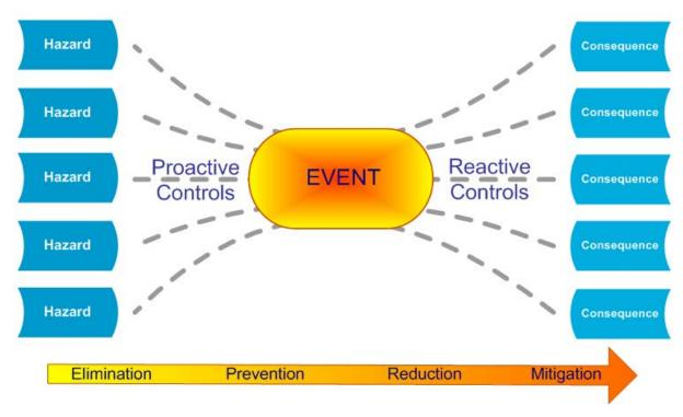
Figure 5 – Schematic Representation of a Bowtie Diagram
