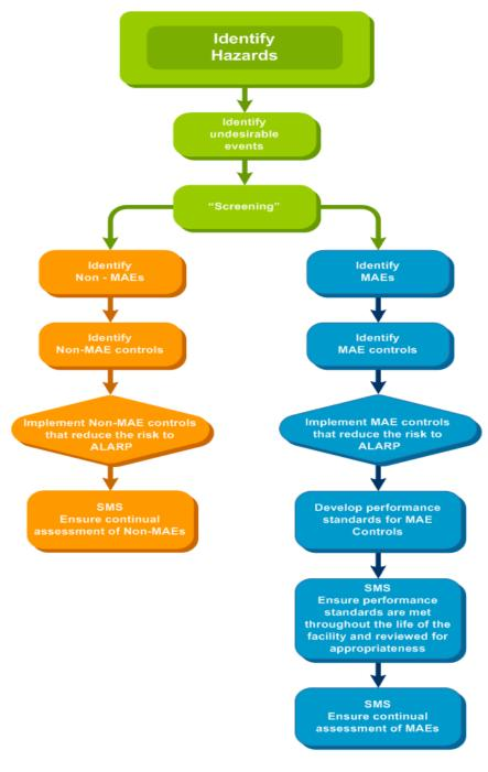
Figure 4 - MAE and non-MAE control measures
