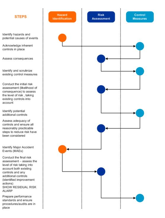
Figure 3 – The FSA process
