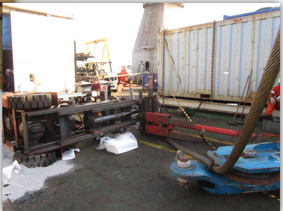
Toppled forklift (manned at the time)
