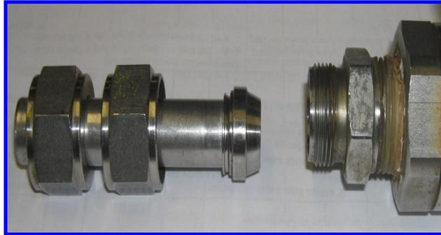
Potential failure will not be evident without adequate post-assembly inspection and may not become apparent for a number of years due to a range of factors including operating conditions and the material of the tube and fittings. Even during regular pressure testing, it is not uncommon for these 'compromised' fittings to pass the initial and subsequent tests prior to the main failure event.
