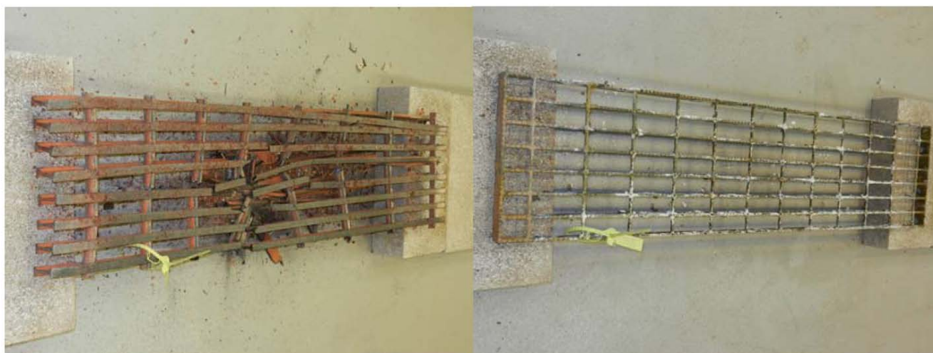
Figure 1 FRP (left) and steel (right) gratings post dynamic testing.
