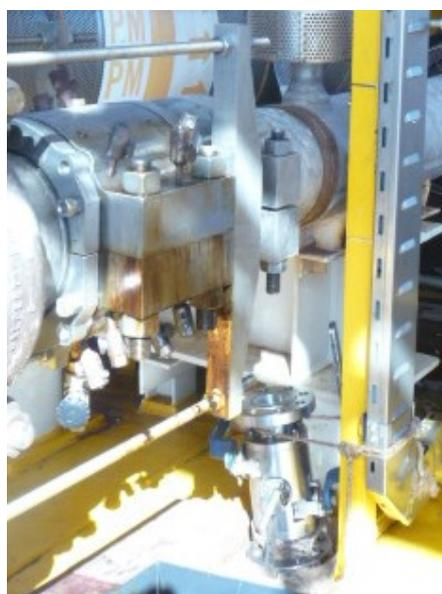
Failed hydrocarbon test header with engineered temporary clamp
