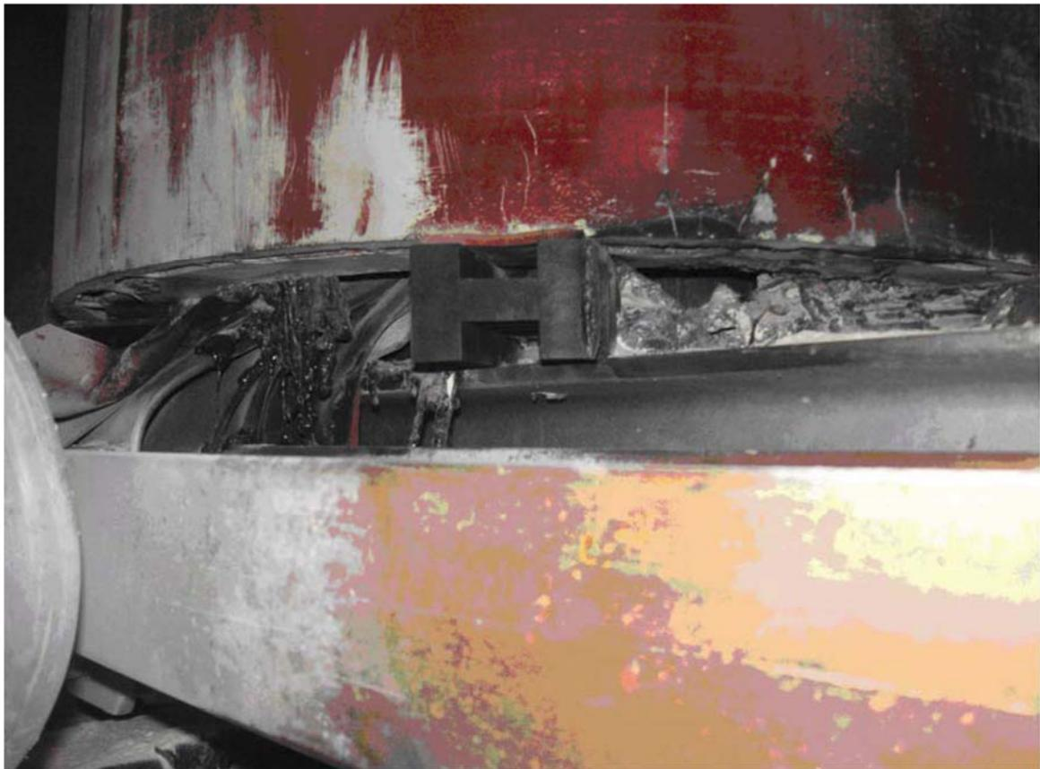
In this incident, the transformers had not been correctly rated. Transformers intended for use with inverter drives should be rated for the additional heating effects imposed by harmonic currents resulting from the non-linear nature of switched and unbalanced loads.
