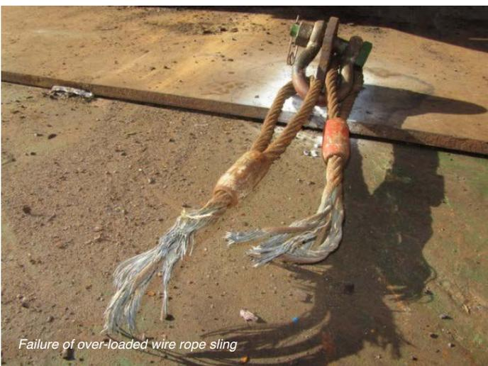
Failure of over-loaded wire rope sling
