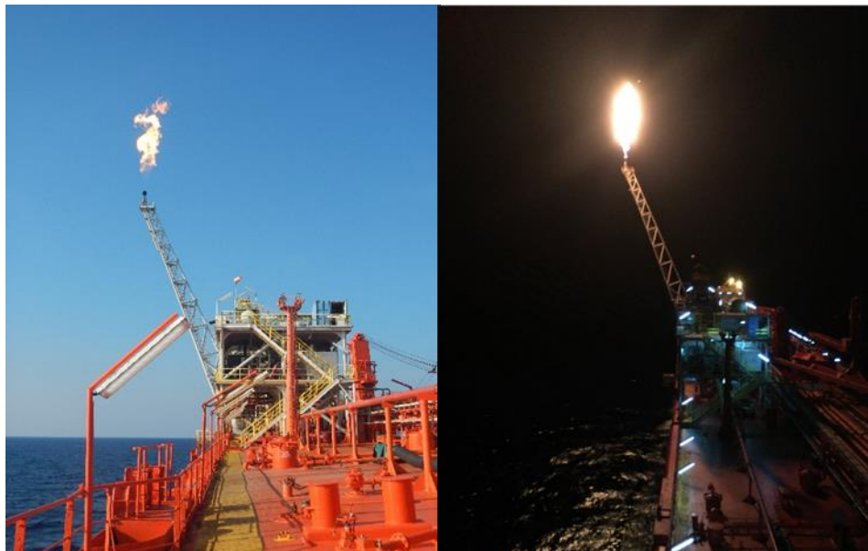
Figure 7-2 Galoc FPSO (Philippines) Flaring Day (left) and Night (right) at ~15 MMscf/d
