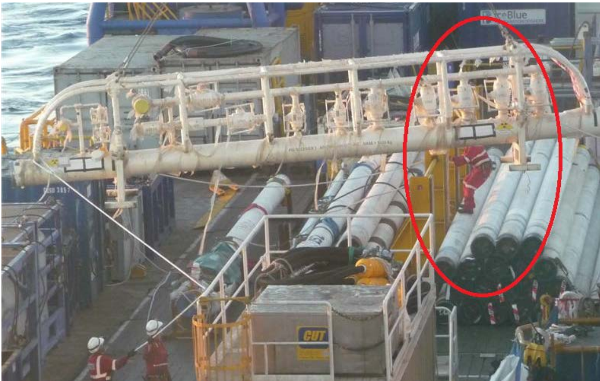
Figure 2 – Pipe rack location impedes lifting operations
