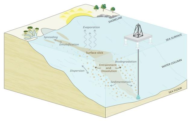
Figure 4 Weathering processes conceptual model
